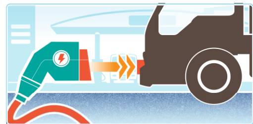
Figure 11: The EVSE plug connects with the EV receptacle to transmit power over a conductive system
